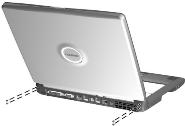
Figure C-2. Torx T8 M2.5 × 7.0 Screw Locations
