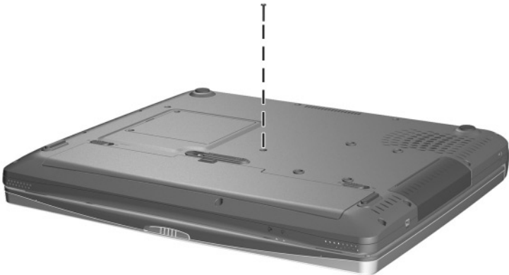
Figure C-8. Torx T8 M2.5 × 16.0 Screw Locations
